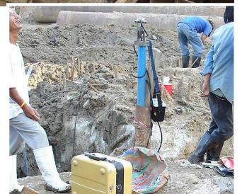
Fig.8 Example of application Measure the lateral movement of pile by inclinometer during Static lateral pile load test.
