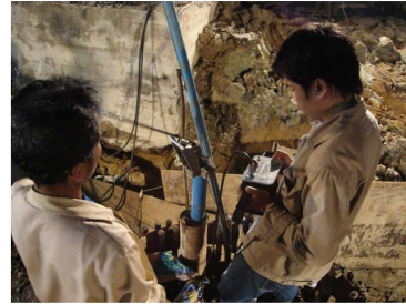
Fig.8 Example of application Measure the lateral movement of pile by inclinometer during Static lateral pile load test.
