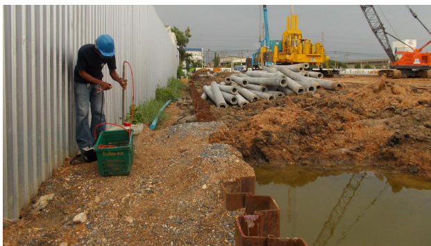
Fig.7 Example of application measure the lateral soil movement caused by pile installation by inclinometer. Behind the fence, have a properties required to protect.
